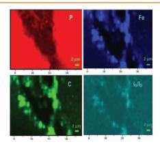
A local visualization study of the influence of impurity phases on carbon coating for LiFePO<sub>4</sub> is presented. It is demonstrated that a phosphorus-rich phase has an inhibiting effect (or no positive catalytic effect) on carbon formation, while ironrich phases (mainly iron phosphides) promote carbon growth by contributing to more carbon deposition and a higher graphitic-carbon content.
